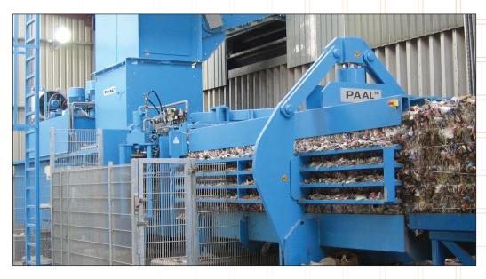
Kadant PAAL's DOKON fully automatic channel baler's unique design makes the PAAL DOKON baler a powerful, efficient bale press with horizontal twine tying system. The PAAL DOKON baler provides a pressing force of 90 to 218 tons and offers a bale format of 32" x 44" or 44". The combination of high pressing force, independence from the cutting and compressing process, and patented pre-press setting combined with individual channel adjustment lead to high quality baling results.
